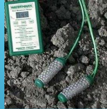
Electrical Resistance Blocks
