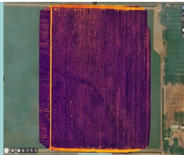
Drone infrared thermal test conducted on a field with buried drip to determine irrigation distribution and evapotranspiration uniformity.
