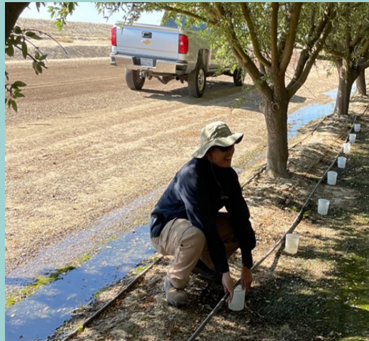
Kevin Young-Lai (Solano RCD) conducting flow measurement tests on dripline.
