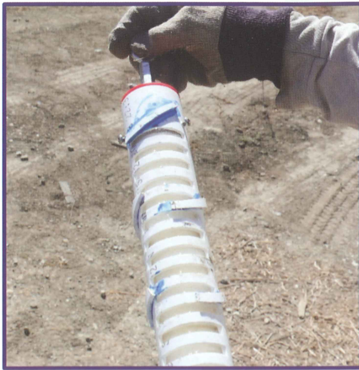
Figure 3: Prototype dry PAM applicator for pressurized irrigation systems (left) and PAM cartridge that inserts into the applicator (right).
