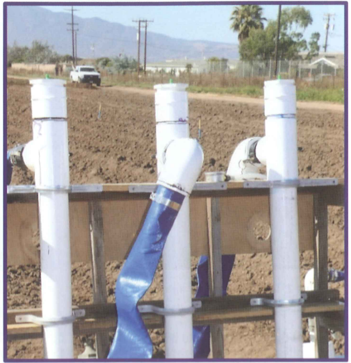
Figure 3: Prototype dry PAM applicator for pressurized irrigation systems (left) and PAM cartridge that inserts into the applicator (right).
